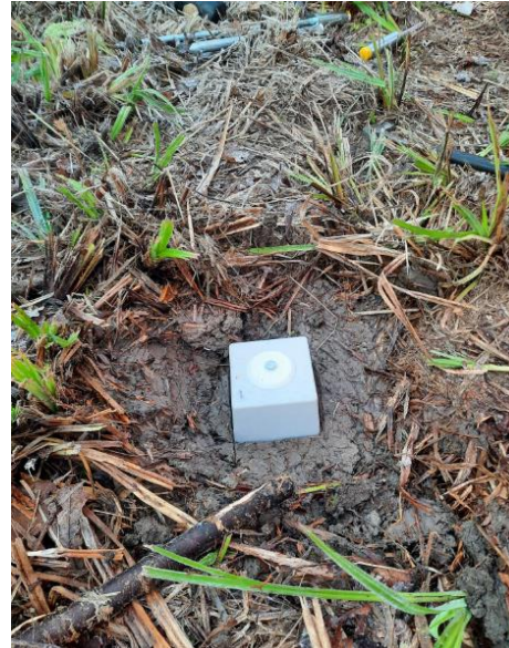
Survey anchor for Soft Ground to mitigate seasonal variations Depth can vary between 0.4m and 1m
