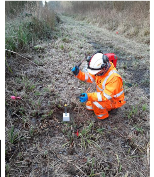
Survey anchor for Soft Ground to mitigate seasonal variations Depth can vary between 0.4m and 1m
